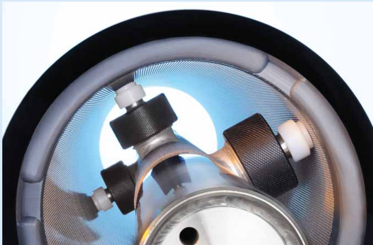
Amiad's scanning nozzles focus backflush on 1 sq in. of screen at a time, making backflush more effective and water efficient.
