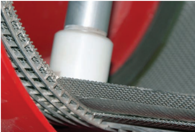
When a pressure differential is reached, the suction nozzle of this automatic self-cleaning screen filter opens and filter cake is pushed off of the screen by the focused back flush of water into the nozzle.
