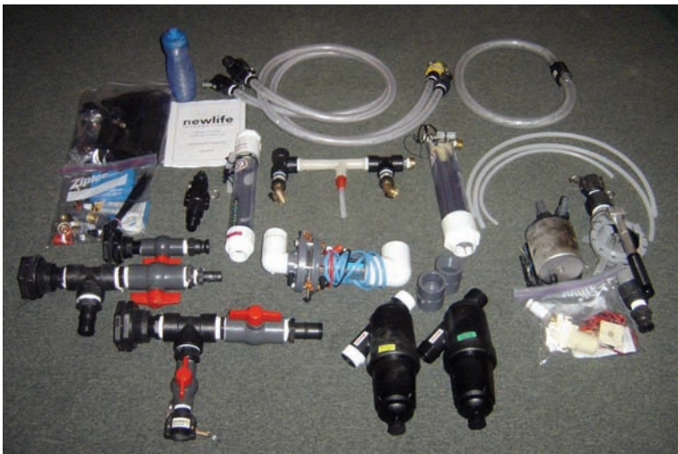
McGuire's water purification system includes two degrees of filtration and a sidestream chlorination system that uses electricity and table salt to disinfect entire tankfuls of water.
