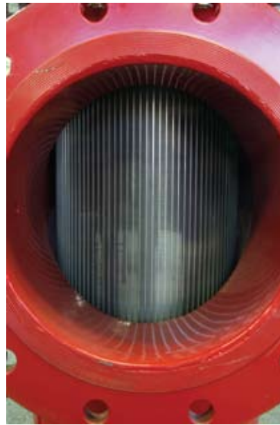
Four layers of woven stainless steel screen and a highly effective back flush system keep this filter clean and effective as a safeguard against zebra and quagga mussels. (Photo: Amiad Filtration systems)
