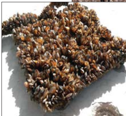
When juvenile quagga mussels settle down, colonies form quickly, with devastating results, like these smothered sampling plates from Parker Dam, which holds back Lake Havasu. (Photo: US Bureau of Reclamation)
